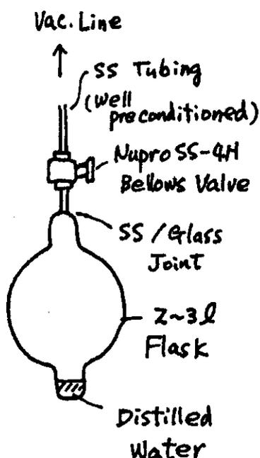
2) Attach a well treated (conditioned) all stainless steel bellows valve (e.g. Nupro SS-4H).
